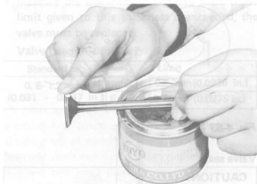
Fig. 4-69 Applying lapping compound to valve face
