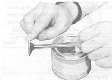
Fig. 4-69 Applying lapping compound to valve face
