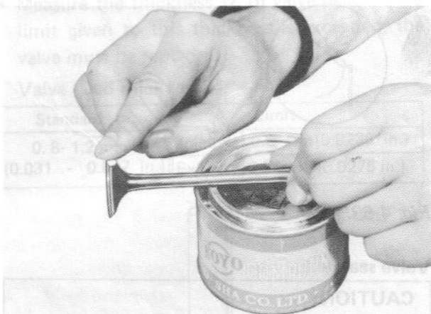
Fig. 4-69 Applying lapping compound to valve face
